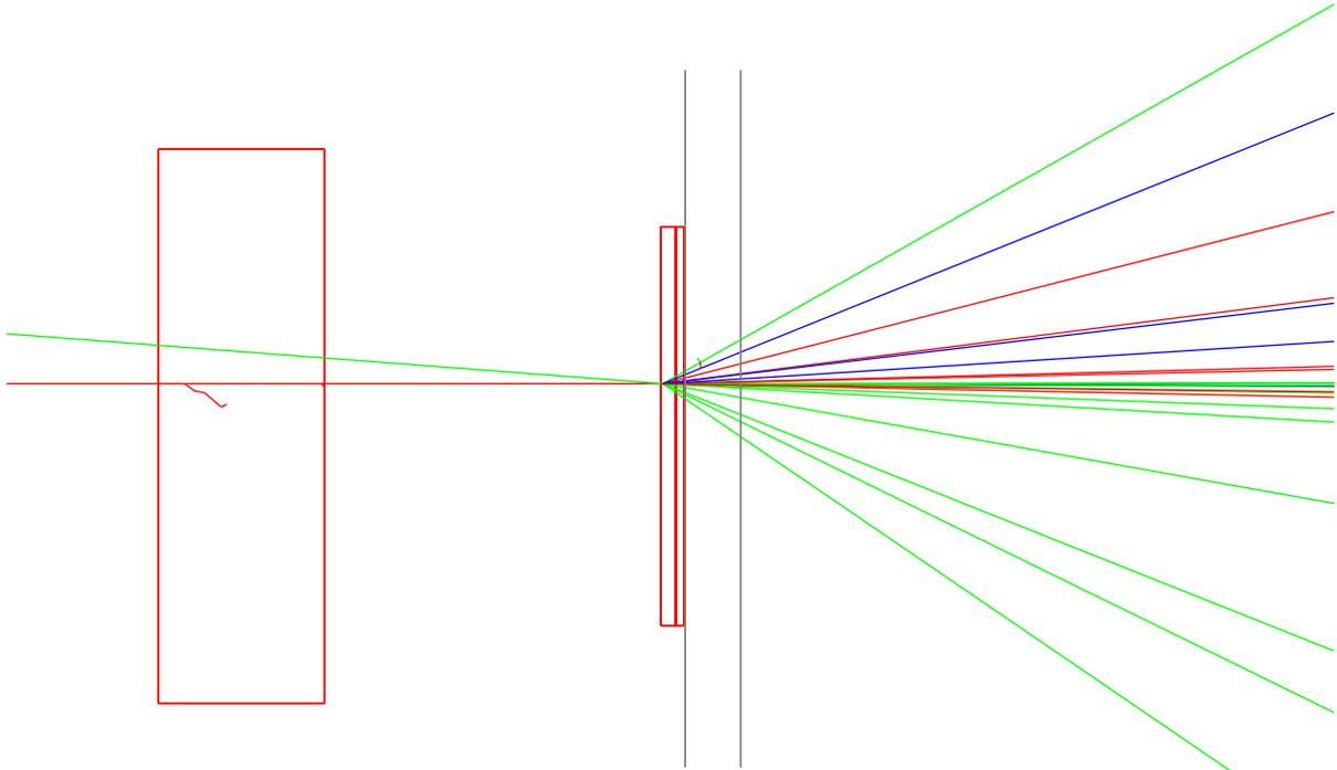
Figure 2: Pixel detector schematic layout: from left to right, plastic cover ( $3\text{ mm}$  thick), silicon sensor ( $280\ \mu\text{m}$  thick), front end read-out chip ( $150\ \mu\text{m}$  thick), printed circuit board ( $1\text{ mm}$  thick). A simulated hadronic interaction in the sensor is shown.
