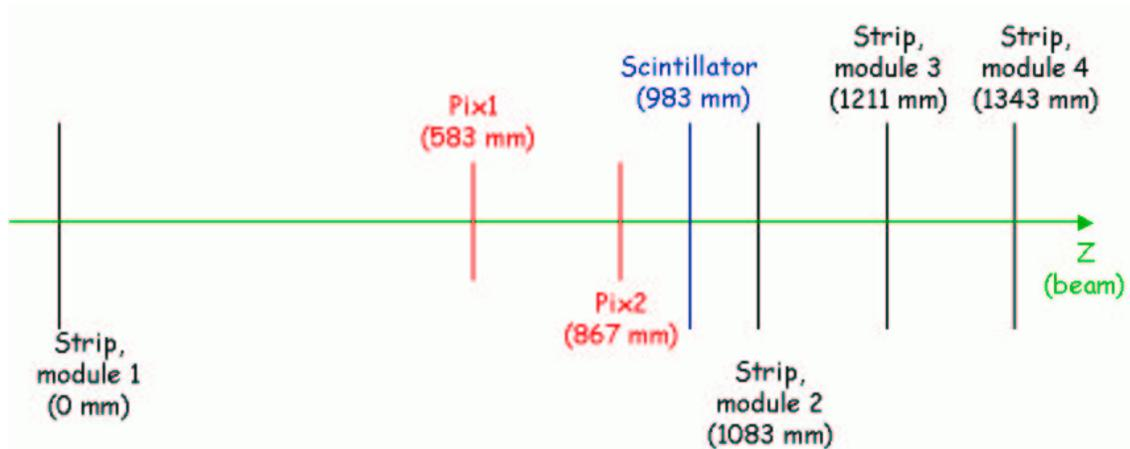
Figure 1: Pixel test-beam setup.
