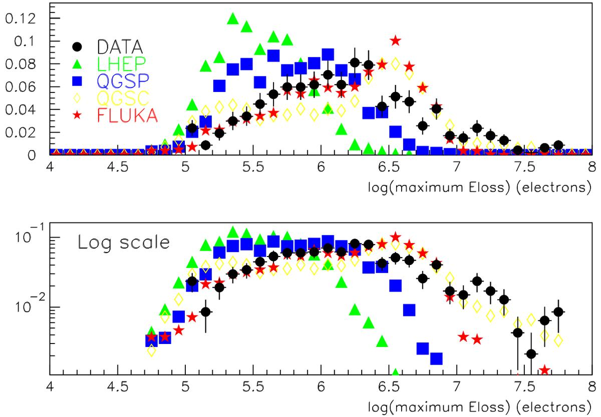
Figure 10: Maximum charge in a single pixel of the cluster.
