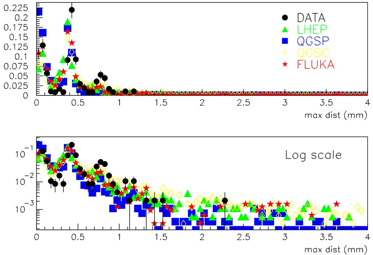
Figure 8: Distance of the farthest pixel of the cluster from the cluster barycenter.
