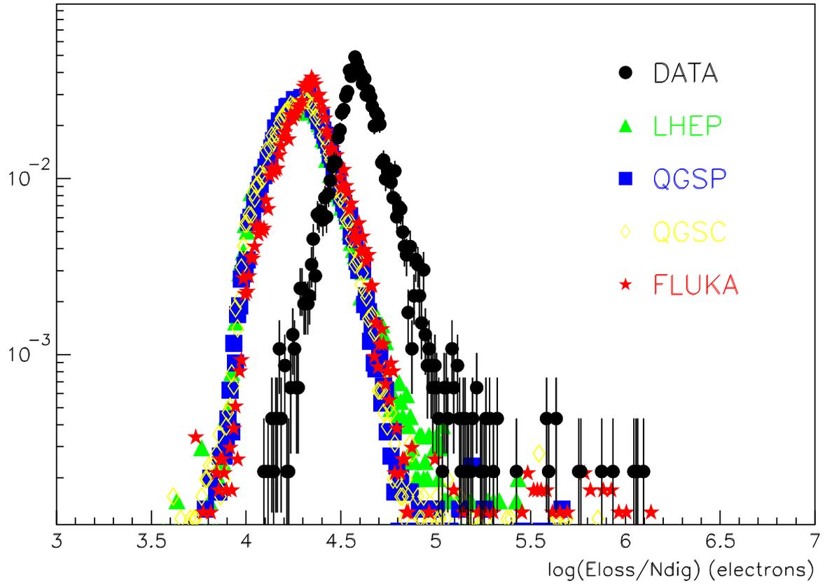
Figure 3: Released energy in the pixel sensor normalised to the number of digits in the cluster for events originating in the plastic cover.
