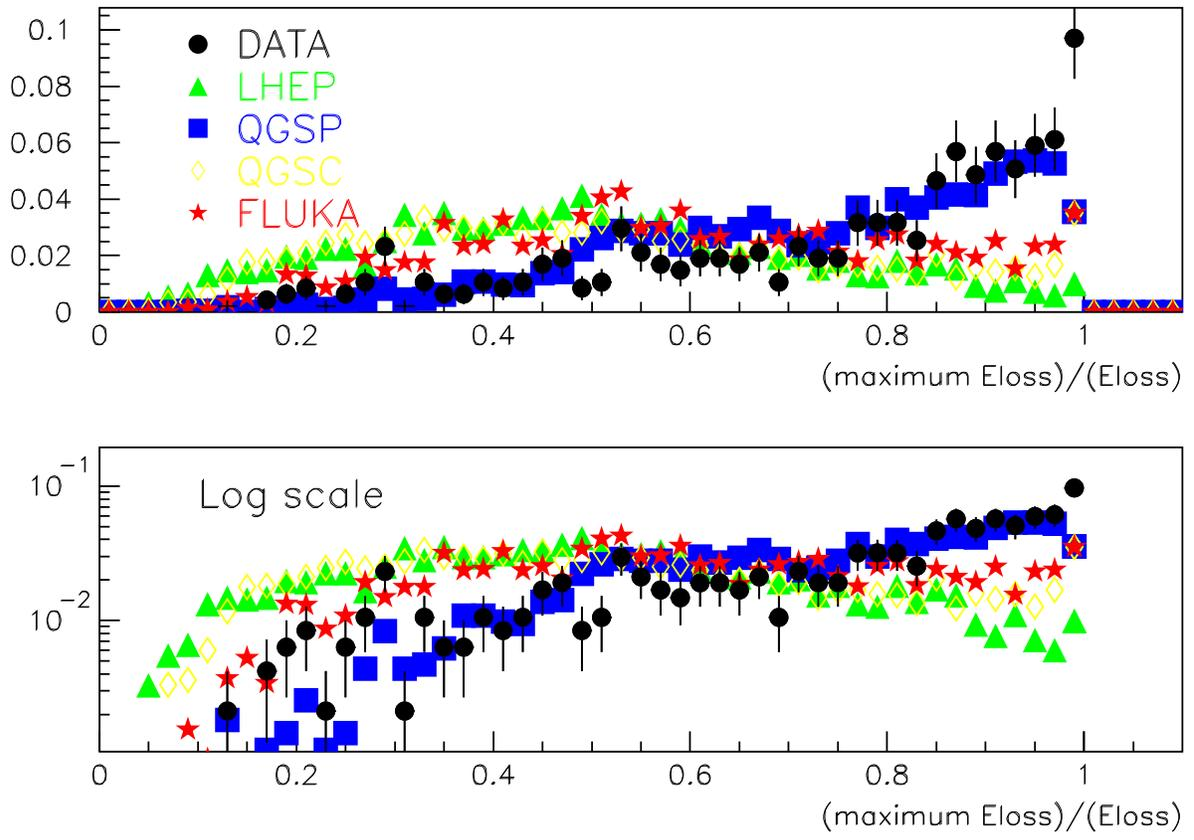
Figure 6: Maximum energy in a single pixel of the cluster divided by the total cluster energy.
